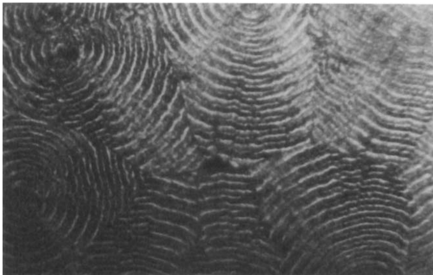
Figure 1a. Ringed spherulites formed during cold crystallization of 9-DDA-9. Magn. 320x.
